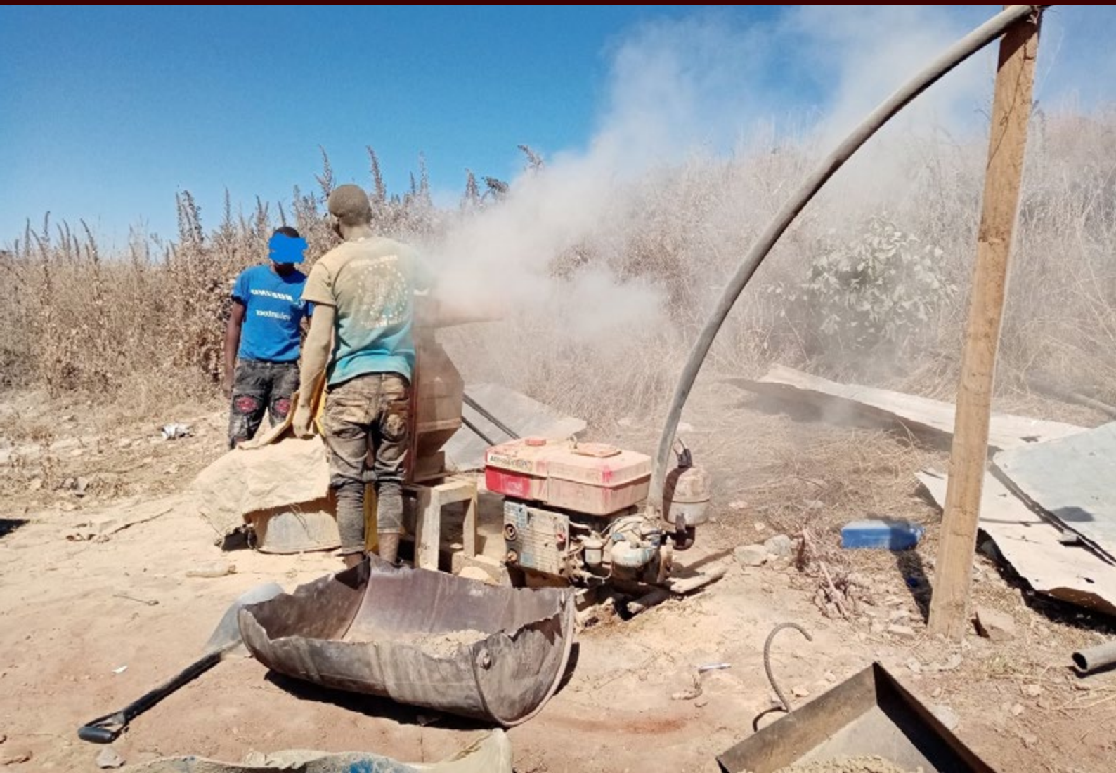
Figure10: Crushing gold ore using diesel-powered grinding machinery at Masase, Mazowe. Over 50 privately owned gold mills are located at Masase camp (Picture Credit: CNRG)
