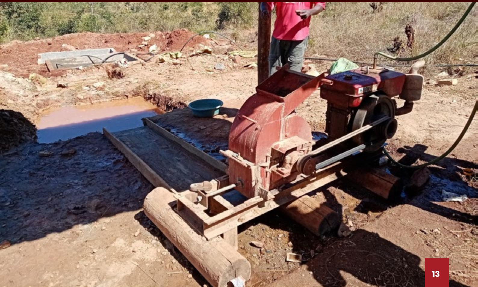
Figure 2: One of the private, unregistered gold mills (diesel-power grinding machine) on the boundary of Redwing Mine claim. ASMiners take their ore to these mills (Zviguruguru) where the gold produced is hardly accounted for.
