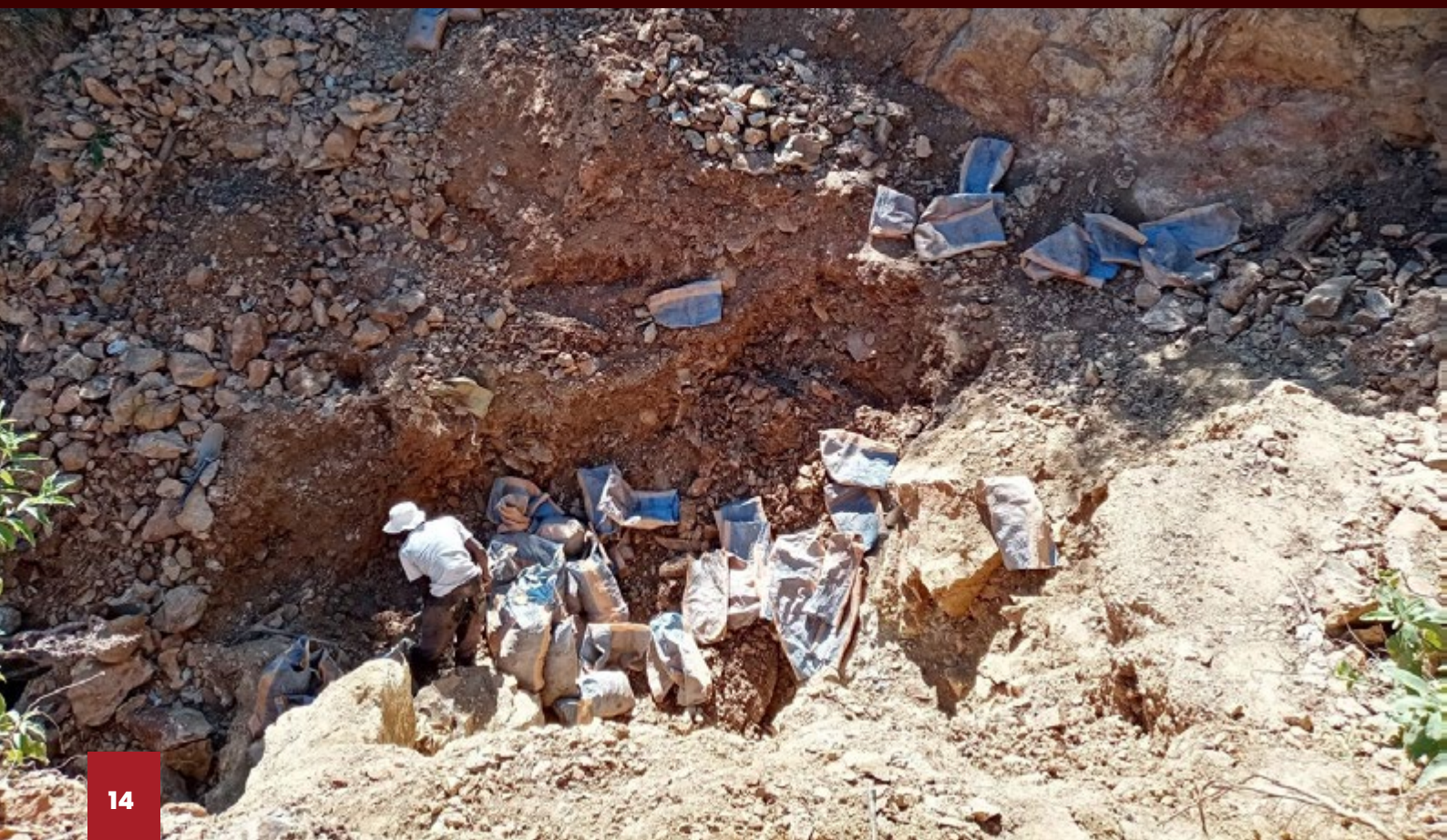
Figure 3: Artisanal miner scoops ore from a pit into sacks or bags in Penhalonga mountains within the Redwing Mine claims. The bags are carried either to PRM mill or other private mills.
