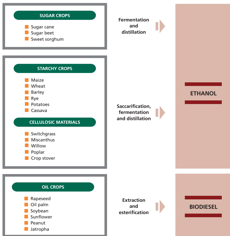
FIGURE 6 Conversion of agricultural feedstocks into liquid biofuels
